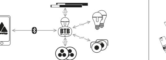
Please power on the light. Hold down the power button for 3 seconds until the light flashes blue. If you are using a LunaBulb as BTB you must use a White Remote (ARC3) to active BlueMode. In the AsteraApp press „Manage Bluetooth Bridges“, then „+“ and follow the instructions on screen to connect. The light which is connected as BTB shows a small Bluetooth icon in the display.
